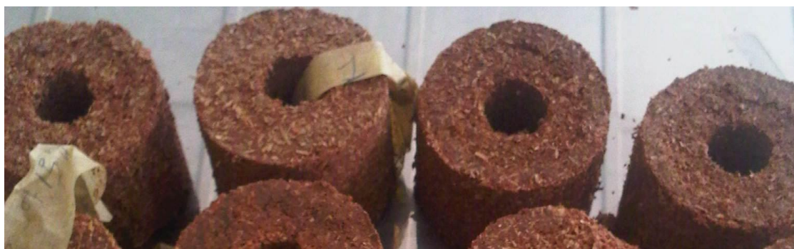
Plate 1: Cylindrical briquettes made from Gmelina sawdust
